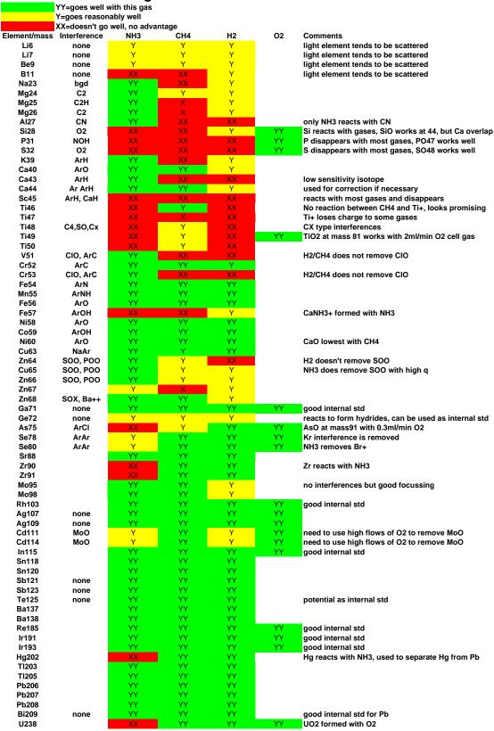
The Most Common Interferences in ICP-MS
